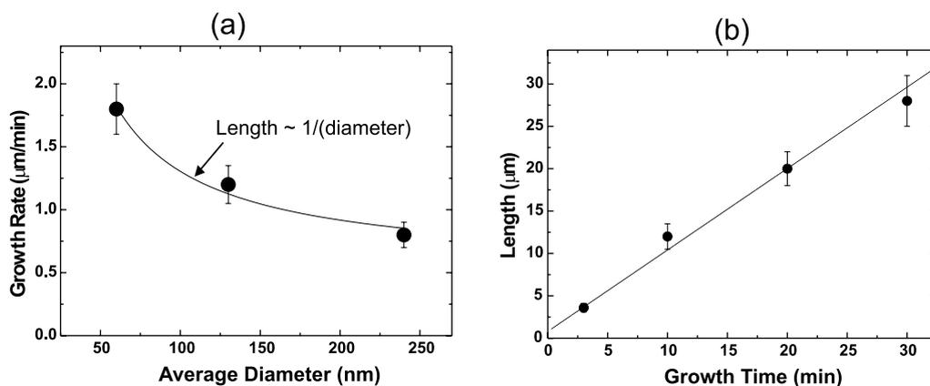
Fig. 2. Dependence of CNT growth on the average diameters and growth time: (a) The growth rate of CNTs as a function of average diameter. The data points are fitted by an inverse function of average diameter shown as a curve. (b) The length vs. the growth time for the CNTs with a diameter of 130 nm.
