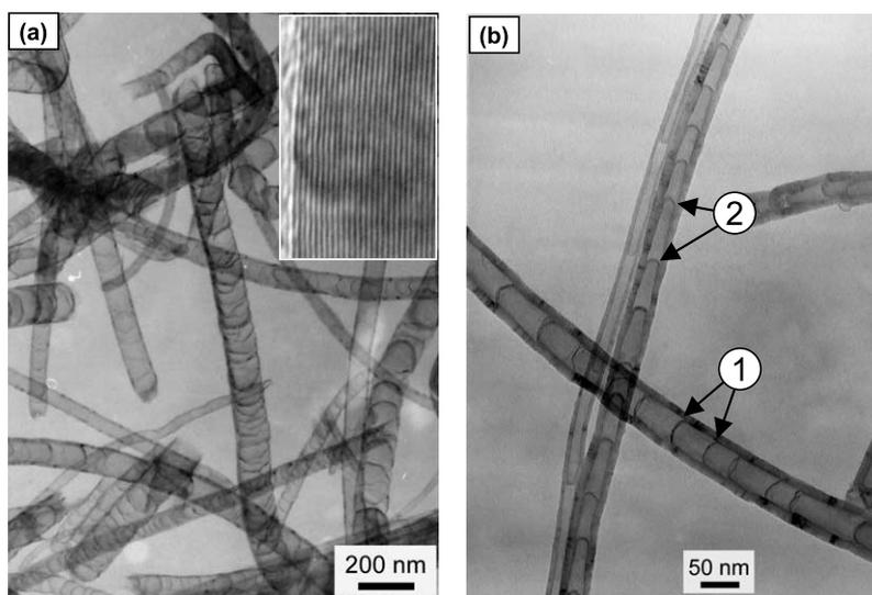
Fig. 3. TEM images showing that all CNTs have bamboo-shaped structure: (a) TEM image for bamboo-like structured CNTs, revealing the closed tips without encapsulated Fe particles and compartment layers with a curvature directed toward the tip. The inset in Fig. 3a shows that high-resolution TEM image, revealing that graphite sheets have a good crystallinity. (b) TEM image showing that compartment layers appear at a longer distance as the diameter of CNTs decreases (see arrows ① and ②).
